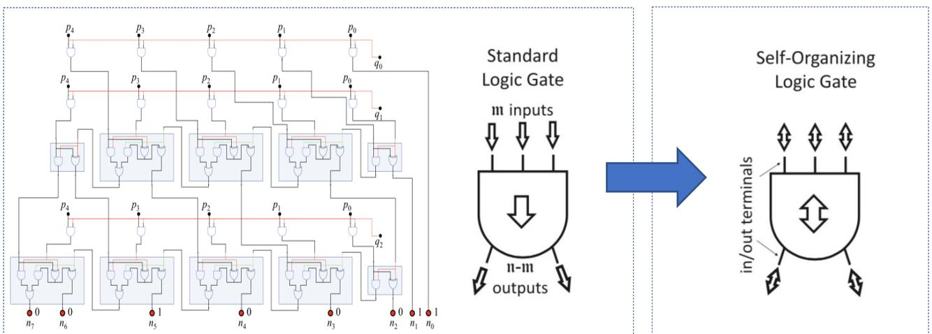
A traditional Boolean circuit using logic Gate for prime factorization
